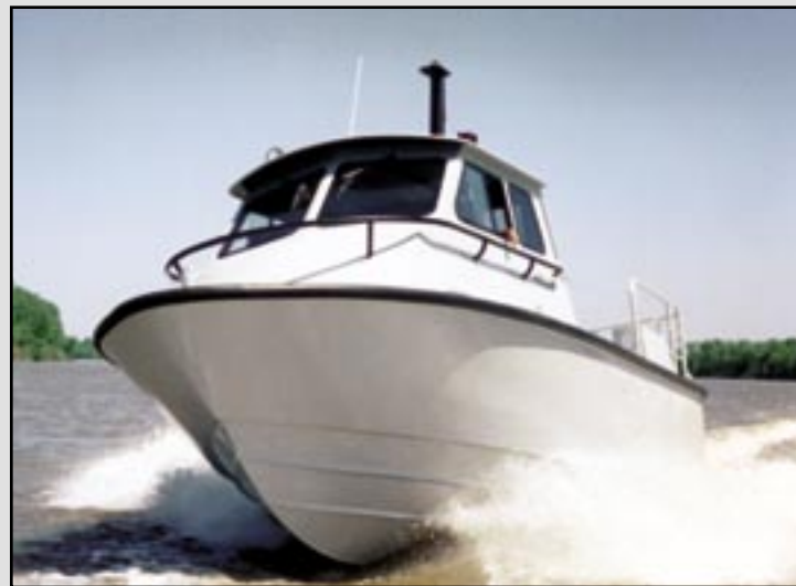
All Dauntless Models Feature Wide Chines, Lifting Strakes And Flared Bows
